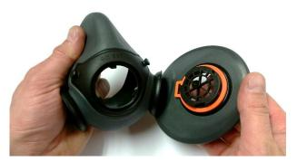
Detach the filter holder from the mask by turning it a  $\frac{1}{4}$  of a lap.
